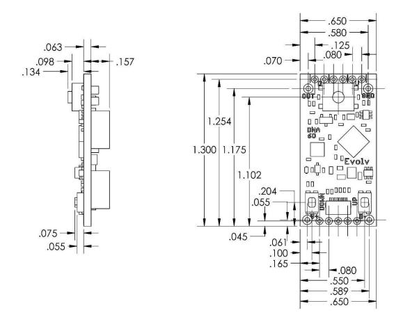
Evolv has 3D models of the DNA 60C available on their website in IGES, STP and Solidworks format.
